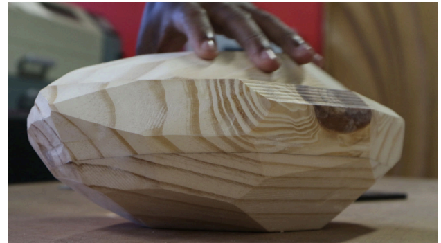
Figure 5: Two part CNC milled prototype in Medellin
