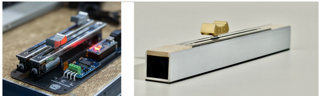
Figure 5. Haptic fader: version for the workshop at the Ljudmila Science and Art Laboratory (left) and for the Ableton Loop Festival (right).
