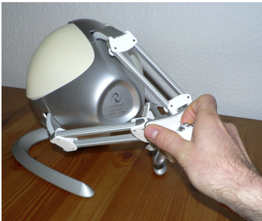
Figure 1. NovInt Falcon haptic force-feedback device.
